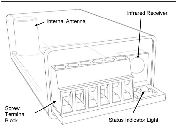
**Figure 3: TX10K-LP-S Transmitter**
